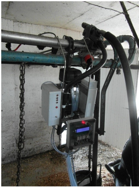
Fig. 2. Quarter milking cluster equipment (design version 3) (source: author's own photograph)
