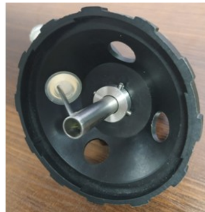
Fig. 4. Measuring module equipped with a single thermistor (source: author's own photograph)
