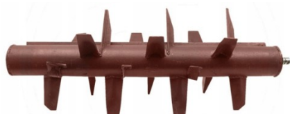
Fig. 2. Spreading drum of the Fortschritt T-088 technological trailer
