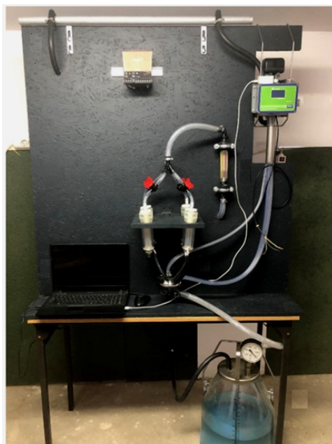
Fig.3. Laboratory station for testing a quarter milking system controlled by temperature sensors
