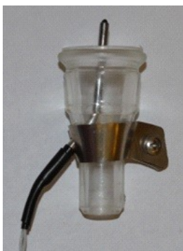
Fig. 2. Method of installing a temperature sensor in an inspection glass of a teatcup
