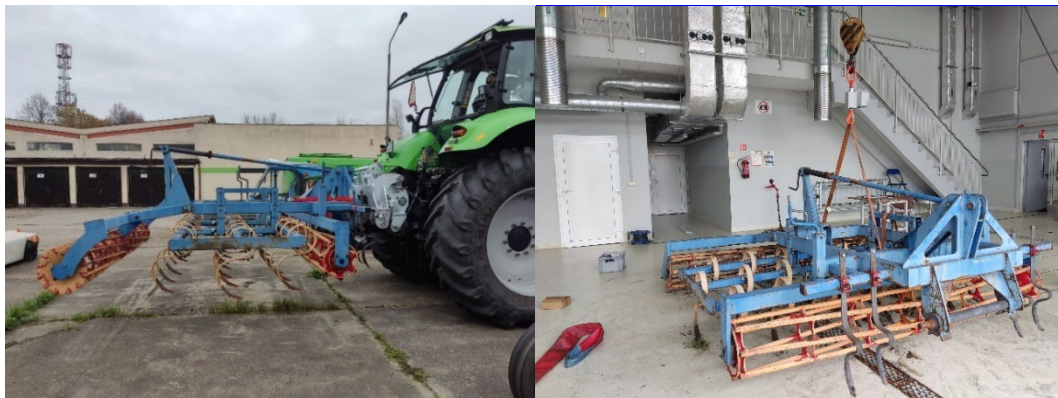
Fig. 2. The cultivation unit suspended, weighed and leveled on the measuring frame (left) and the unit mass measured in a conventional way (right).
