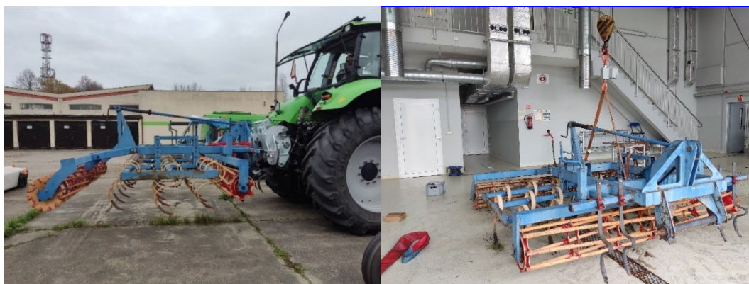
Fig. 2. The cultivation unit suspended, weighed and leveled on the measuring frame (left) and the unit mass measured in a conventional way (right).
