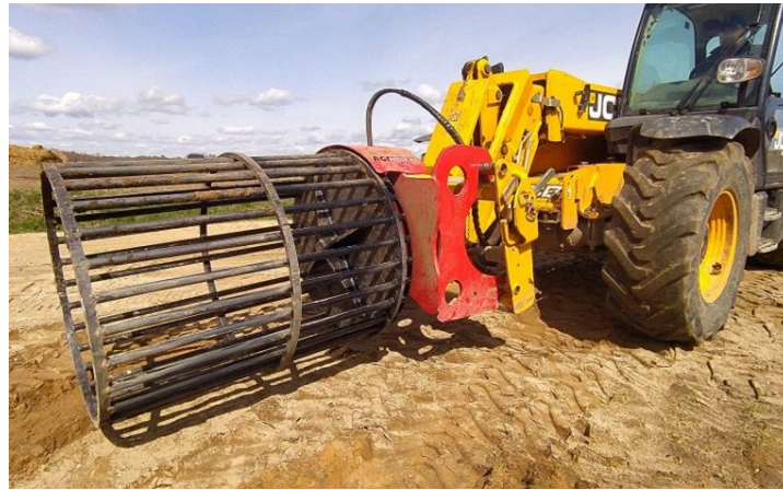
Fig. 3. Agrimet's stone point collection device [32]
