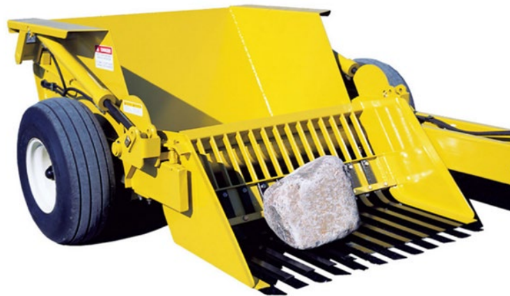
Fig. 4. Degelman stone collector [33]
