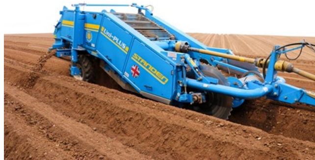
Fig. 14. Standen UniPlus Stone and Clod Separator [47]
