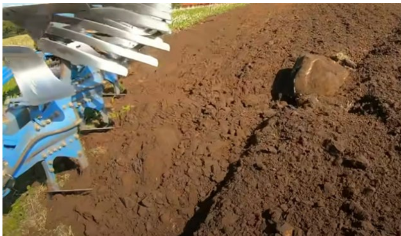
Fig. 1. Lemken rotary plough with hydraulic protection for each body. Source: Authors
