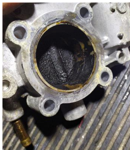
Fig. 4. Contaminated engine throttle. Source: (Author's own work)
