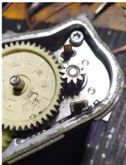
Fig. 3. Hyundai Tucson 1.7 CRDI – sheared teeth preventing engine operation. Source: (Author's own work)
