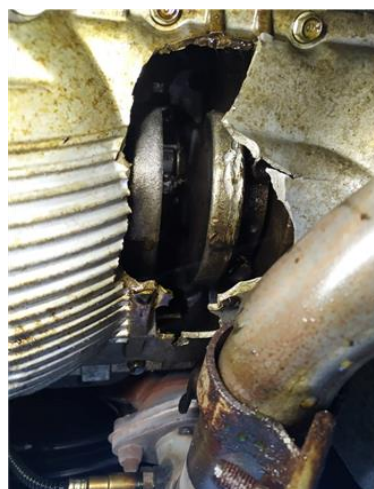
Fig. 7. Connecting rod breakage – Hyundai Tucson 2.0 DOHC engine Source: (Author's own work)
