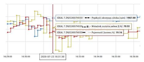
Fig. 6. Chart from AGCO Connect system for three work parameters of combine harvester (source: own work based on [15])
