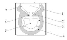
Fig. 3. Scheme of gasification combustion space with manual feeding of billet wood and bio-fuel briquettes (Atmos DC 25 GSE): 1 – space for fuel, 2 – refractory shaped piece with nozzles, 3 – combustion products off take, 4 – combustion products exchanger - water, 5 – after – burning space with ash pan, 6 – secondary air intake, 7 – primary air intake
