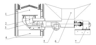
Fig. 1. Scheme of combustion system with bottom fuel supply (Pelling 27): 1 - combustion space with ceramics, 2 - retort burner, 3 - fuel auger conveyor, 4 - ash hopper, 5 - burning air ventilator, 6 - fuel container, 7 - electric motor with gear box
