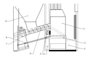
Fig. 2. Scheme of combustion system with self falling fuel supply (Verner A 25): 1 - combustion space with burner, 2 - grate bar, 3 - ash hopper, 4 - burning air ventilator, 5 - heating bar, 6 - fuel auger conveyor, 7 - electric motor with gear box, 8 - grate bars drive, 9 - fuel container
