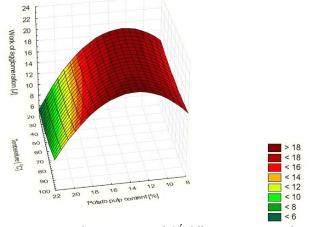
Source: own work / Źródło: opracowanie własne Fig. 3. The influence of material-process factors on the work of agglomeration obtained during the compaction of straw with hard coal and potato pulp
