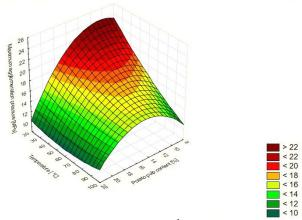
Source: own work / Źródło: opracowanie własne Fig. 2. The influence of material and process factors on the maximum compaction pressures obtained during the compaction of straw with hard coal and potato pulp
