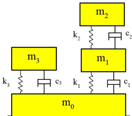
Fig. 1. Three-degree-of-freedom, lumped-parameter biodynamic model of the seated human body vertical vibration [4]
