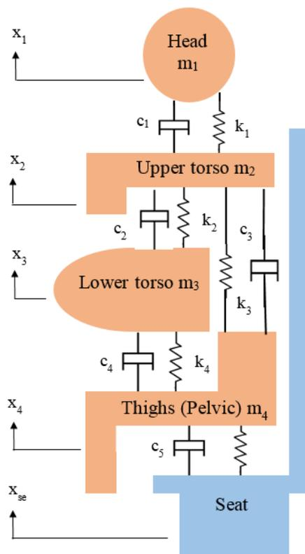
Fig. 2. Wan and Schimmels 4-DOF biomechanical model of human body [8, 16]
