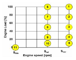
Fig. 4. The NRSC test measurement points [9] *Rys. 4. Schemat testu NRSC [9]*
