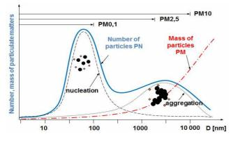
Fig. 2. The idealized relation between the size of particles and their number and mass for exhaust gases from the CI engine [8]
