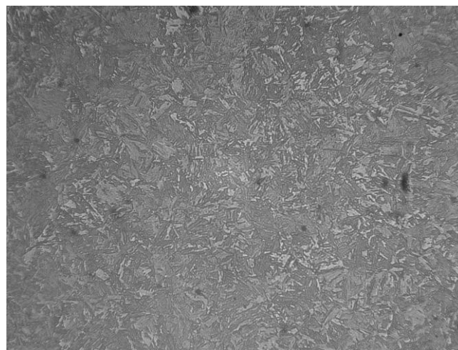
Fig. 2. Microstructure of SSAB BORON B27 steel after austenitising at temperatures: 880^\circ\text{C} – A, 900^\circ\text{C} – B, 920^\circ\text{C} – C and 950^\circ\text{C} – D, quenching in water and low tempering at a temperature of 200^\circ\text{C} \cdot \text{h}^{-1}
