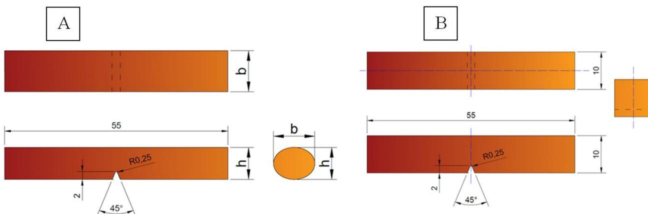
Fig. 2. Preparation and dimensions of samples: A – non-standardized sample, B – normalized sample [11]
