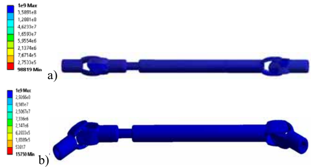
Fig. 9. Amount N of correct cycles of proper operation of the PTO shafts for the case of pulsating positive loads for various values of angle \alpha = 0^\circ (a) and \alpha = 90^\circ (b)
