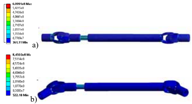
Fig. 6. State of equivalent stresses in the jointed-telescopic shaft for angles of deviation in deriving and derived shafts \alpha = 0^\circ (a) and \alpha = 90^\circ (b)
