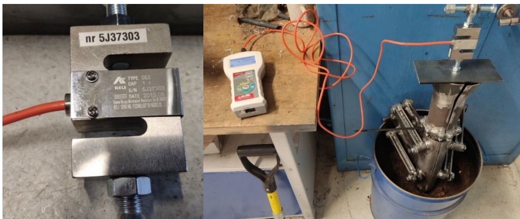
Fig. 5. Force sensor (left), test stand with tool inserted (right)
