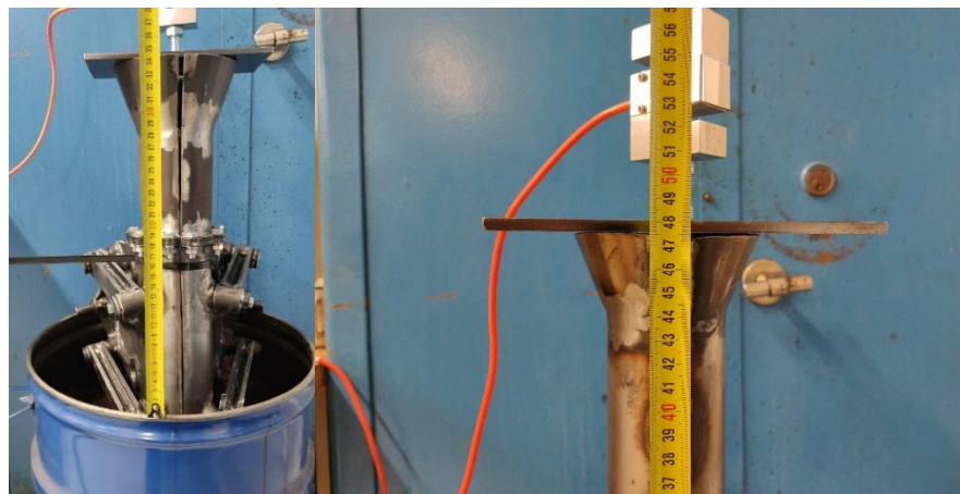
Fig. 6. Measurement of the depth of the tool in the tank after reaching the set force value
