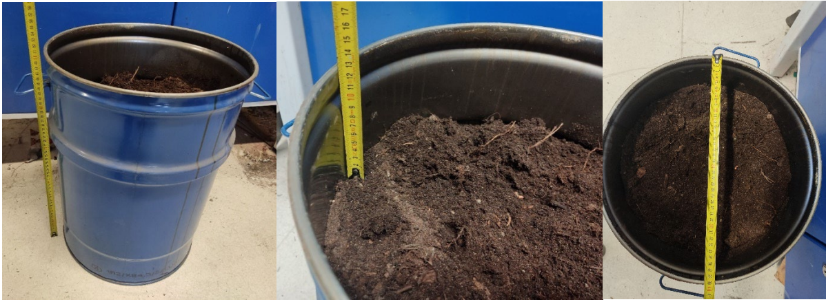
Fig. 4. Tank filled with soil into which the planting tool was inserted
