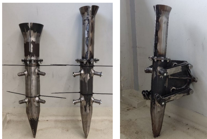
Fig. 3. View of functional models of both versions of the tool, from left: second version (V2), first version (V1), V1 mounted on a frame
